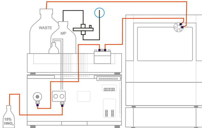
Figure 1. Flow path configuration schematics for passivation of the metal parts in an ALEXYS system. Note that the nitric acid is not going through the Whatman in-line filter, the detector, nor the degasser channels. In case of a dual channel system or gradient set-up the same principle is applied.
